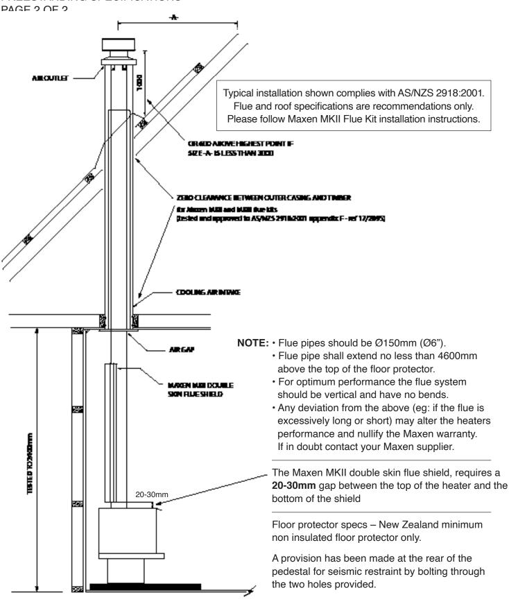
IF INSTALLED IN ACCORDANCE WITH THESE SPECIFICATIONS THE HEATER COMPLIES WITH AS/NZS 2918:2001.
